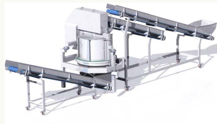
Continuous spin dryer
