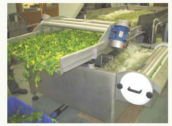
Twin vortex, high capacity washer
