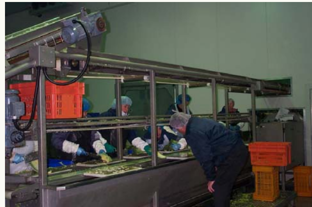
Trim table / conveyor arrangement
