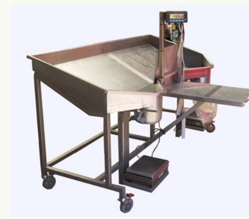
Pack / weighing arrangement
