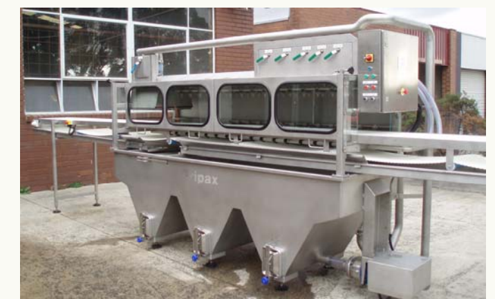
Whole head and bunched produce washer
